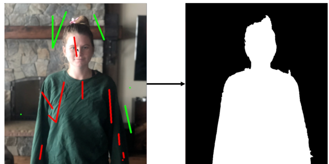
Fig. 3. User marked RGB and accompanying depth map created using implemented watershed algorithm.
