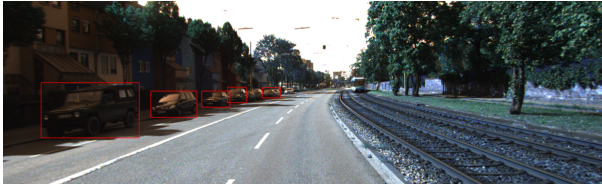
Fig. 8: YOLOv5 identification of cars (red bounding boxes)
