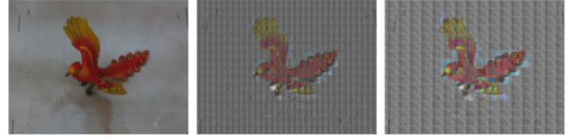
Figure 8. Left: RGB image. Middle: 2.25-bit L\triangledown reconstruction, small blocks. Right: 2.25-bit L\triangledown reconstruction, large blocks.
