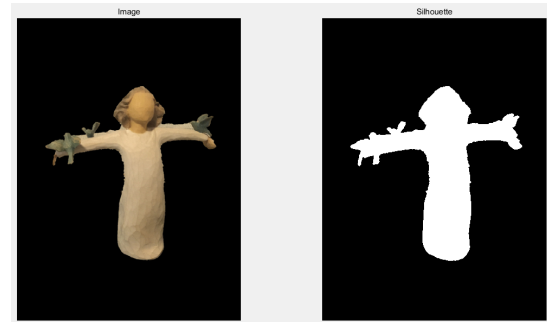
Figure 5. One of the original input images for space carving and its associated silhouette.
