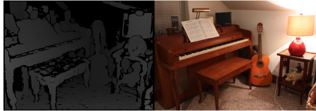
Figure 1. Reconstructed disparity map of a piano from the 2014 Middlebury Stereo Image Dataset.
