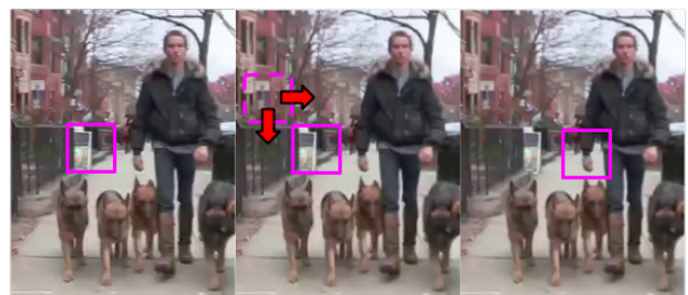
Figure 3: The sliding window method. The image to the left displays the original Yang output for the left hand. The middle image shows the sliding window starting from the top left and moving across and down. A score is calculated for each position. The image on the right indicates the corrected body part which is the position of the sliding window that resulted in the best score.
