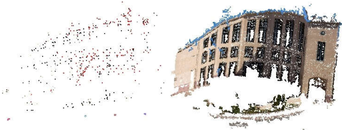
Figure 6. Sparse and dense reconstruction of Scene 2
