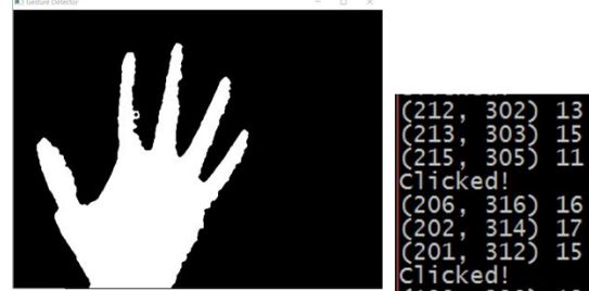
Figure 7: Example of console output. Numbers in brackets are (x, y) coordinates. Number on the right is the number of defects.
