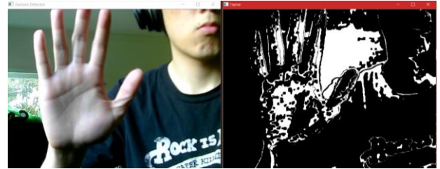
Figure 5: RGB thresholding has both false positives and negatives.
