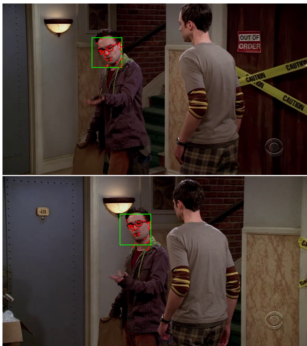
Figure 3: Tracking of a single face throughout a shot. The top image shows the initial detection (green) and the corresponding strong corners (red), and the bottom image shows the corners after tracking and the reconstructed face bounding rectangle.
