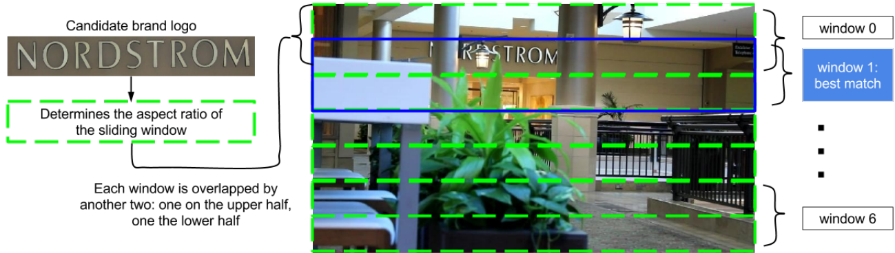
Figure 3: Diagram of our sliding window technique.
